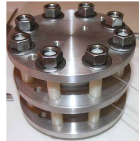
Fig. 4. Photograph of Two-Switch Electrode assembly.
